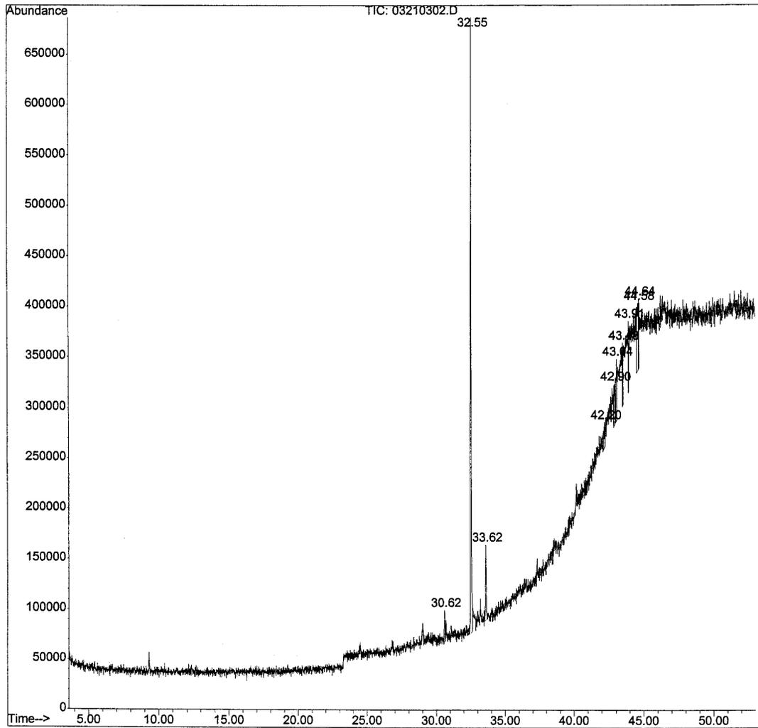
**Figure 16.** Representative GC-MS chromatogram: *Cannabis sativa* extract solvent sample analysis via Volcano<sup>®</sup> vaporization.
