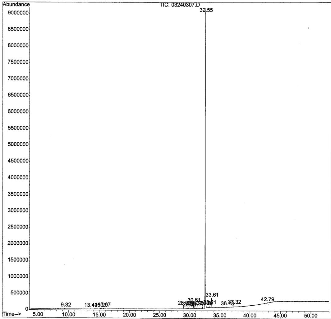
**Figure 17.** Representative HPLC-DAD-MS chromatogram: *Cannabis sativa* extract headspace gas sample analysis via M-1 combustion extraction
