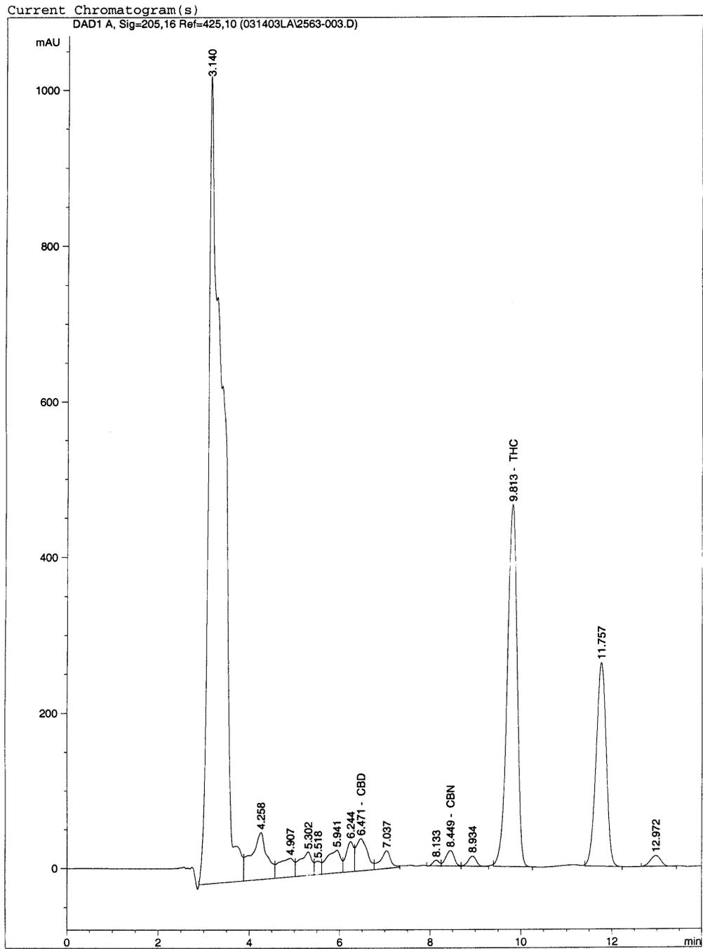
**Figure 10.** Representative HPLC-DAD-MS chromatogram: *Cannabis sativa* extract analysis via Volcano<sup>®</sup> vaporization.
