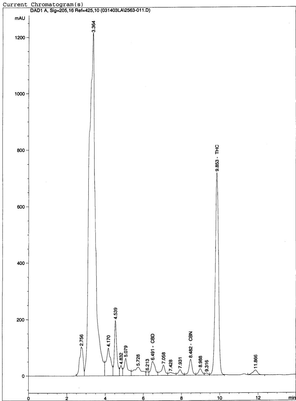
**Figure 12.** Representative GC-MS chromatogram: Method control
